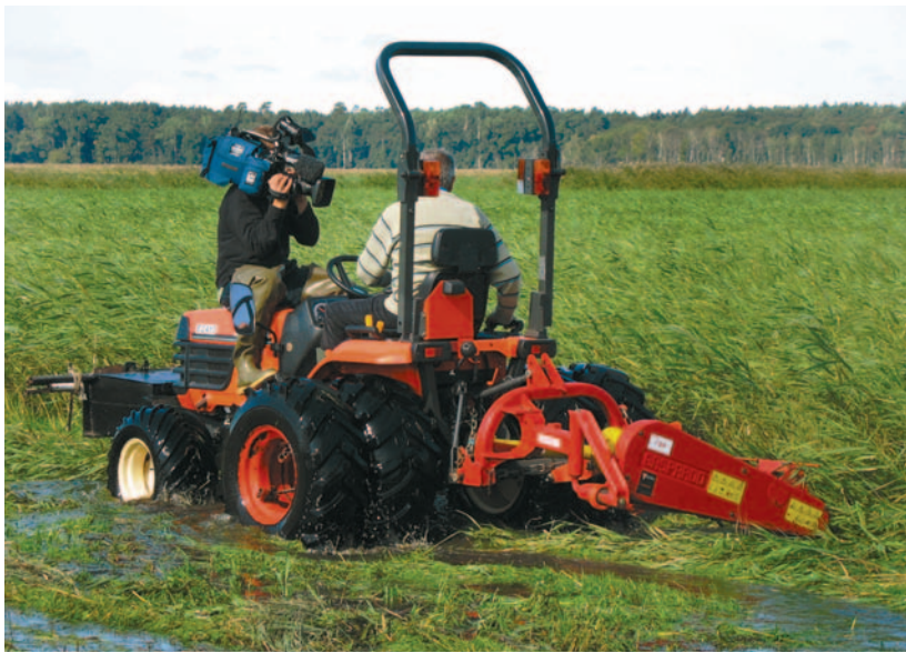
▲ Fig. 4.4.10 ► Seiga harvester used for testing summer mowing at the Rozwarowo Marshes, Poland July 2007 (photo: F. Tanneberger).
