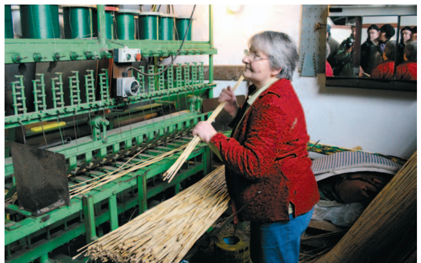
▼ Fig. 5.18 Weaving loom for the production of mats from Common Reed harvested on Schadefähre Island, a former Aquatic Warbler breeding site in Germany, February 2013 (photo: C. Schröder).
