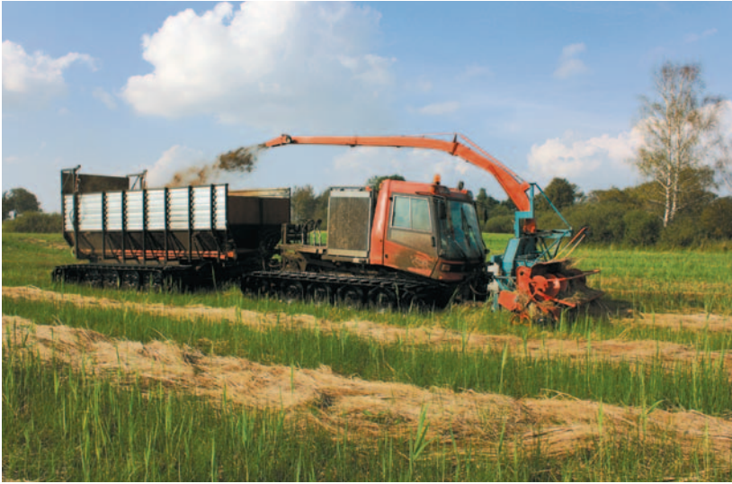
▲ Fig. 4.4.13 Uptake, chopping, and removal of the biomass with chopper and trailer, Peene Valley, Germany, August 2011 (photo: C. Schröder).
